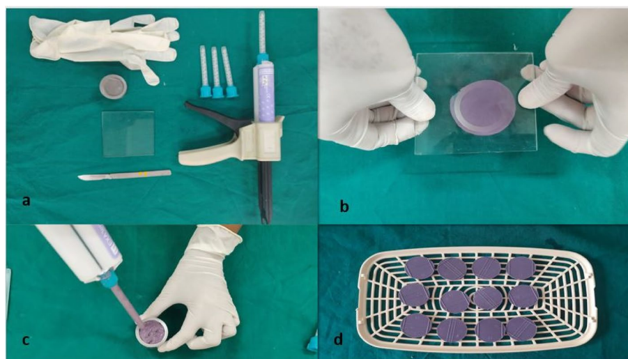
Fig. 3 Procedural steps for making samples- a Armamentarium for the recording of the impression of metal die; b Dispensing of impression material using automixing gun; c Glass-plate is placed on top of the metal die; d VPES impression samples are kept in a tray for washing under running water
