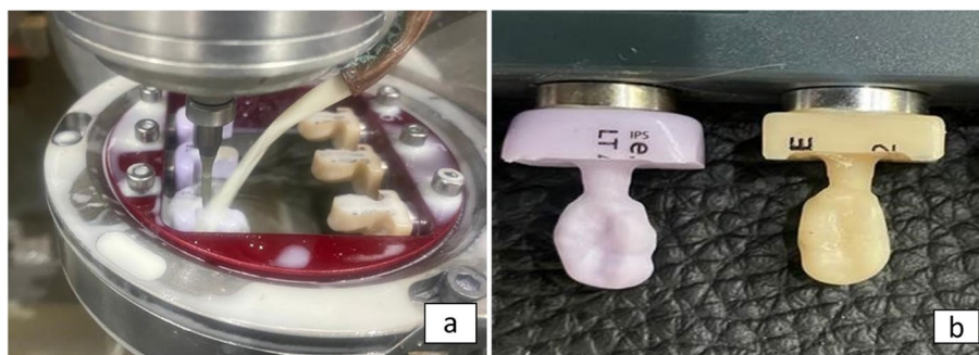
Fig. 5 a & b Milling step by CAD/CAM
