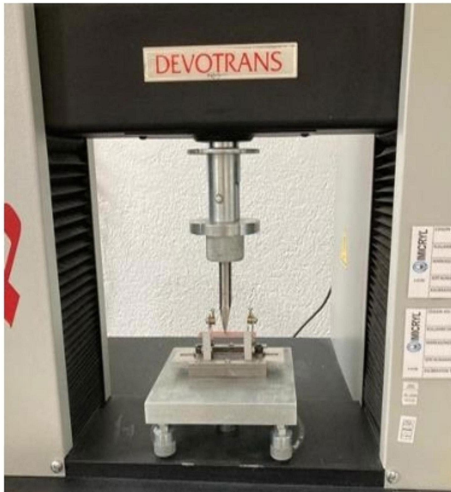
Figure 2. Acrylic specimen loaded on universal testing machine
