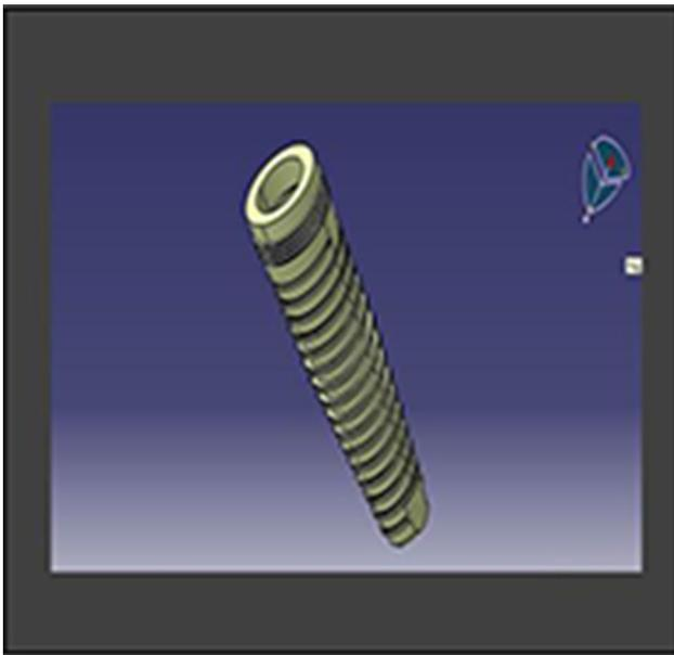
**Fig. 2** Implant CAD model of Dimensions 4×11.5 mm
