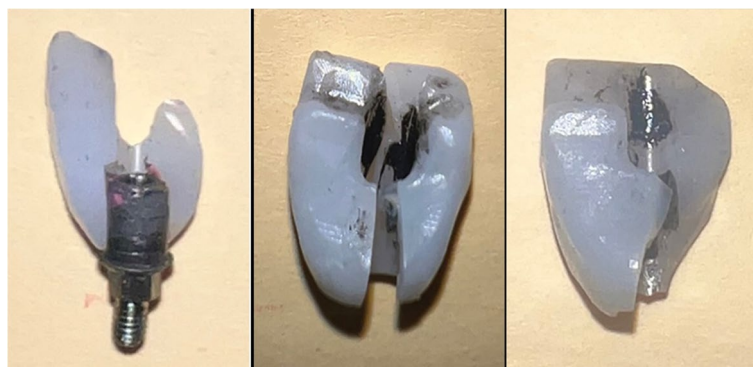
Fig. 7 Modes of failure for all specimens in all groups (note the titanium piece of the abutment apparently intact)
