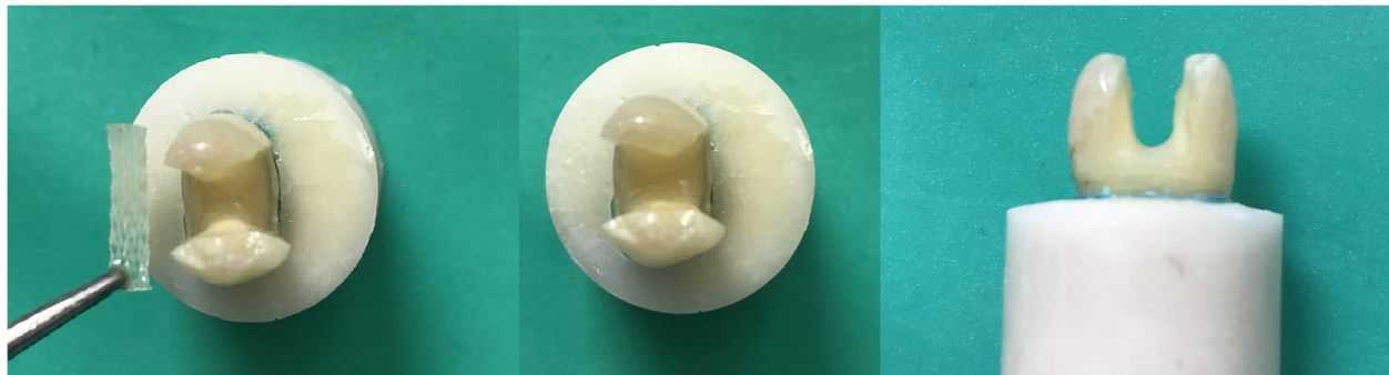
Fig. 2 Fiber placement to the cavity
