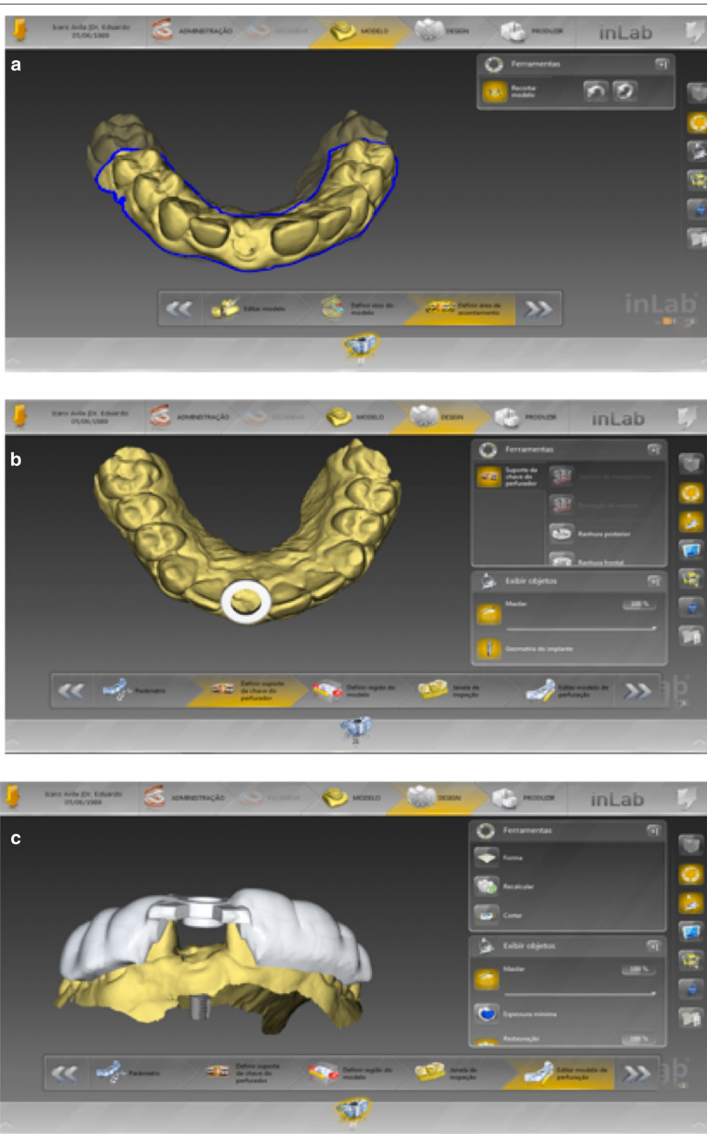
Fig. 1 a Definition of the limits of the surgical guide. b Ring position. c Projection of the final surgical guide
