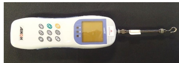
Fig. 2 Digital force gauge. It is used to measure the retentive force along with a hook-shaped traction device that is used to pull palatal palate vertically
