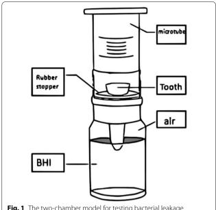
Fig. 1 The two-chamber model for testing bacterial leakage
