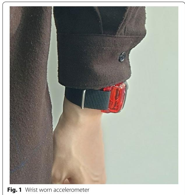
**Fig. 1** Wrist worn accelerometer
