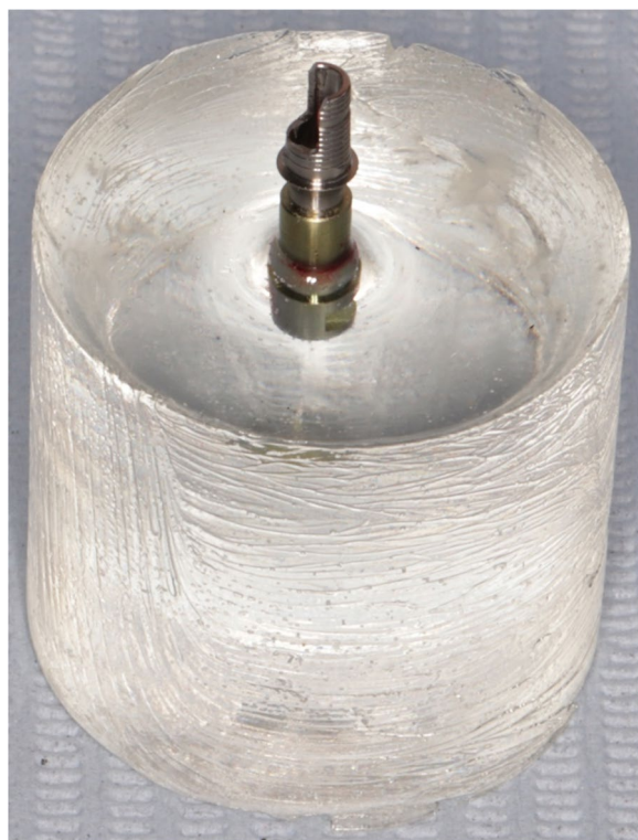
Fig. 2 Group ASC (study group) included angled screw access channel Ti-bases
