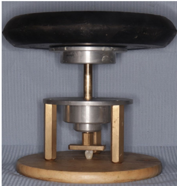
Fig. 5 Load (25 N) was vertically applied for period of 10 min. Caption: Central vertical arm can be only raised for short distance to accommodate height of crown without epoxy resin block
