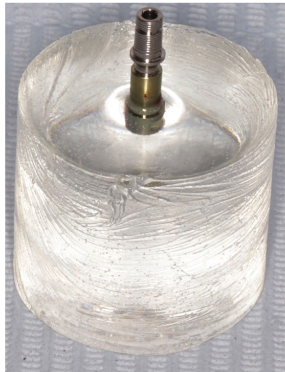
Fig. 1 Group STA (control group) included straight screw access channel Ti-bases
