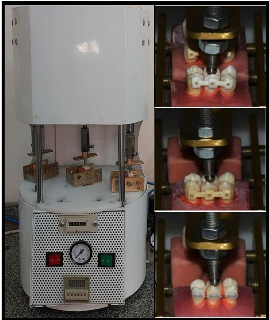
**Fig. 6** The loading cycling machine applied a load on the occlusal of the middle tooth
