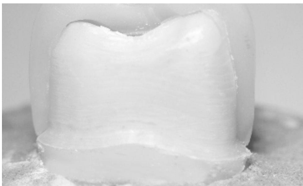
Fig. 3 Stereomicroscopic image showing the fractured specimen with cement attached to the tooth
