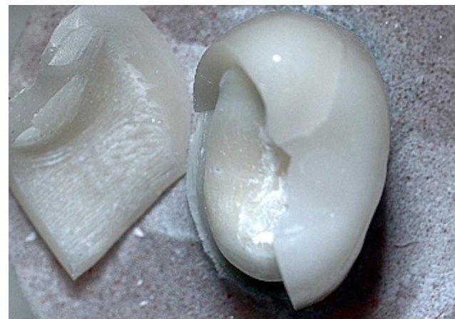
Fig. 4 Stereomicroscopic image showing the fractured specimen with cement remnant on the intaglio surface of zirconia fragment
