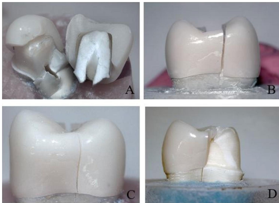
Fig. 2 Stereomicroscopic images showing catastrophic fracture of monolithic zirconia crowns cemented with different cements. A Calibra Universal cement. B RelyX U200 cement. C Panavia SA Cement Plus. D Multlink Speed cement
