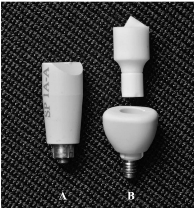
Fig. 1 Investigated scan bodies. (A) One-piece SB, (B) Two-piece HA-SP.
