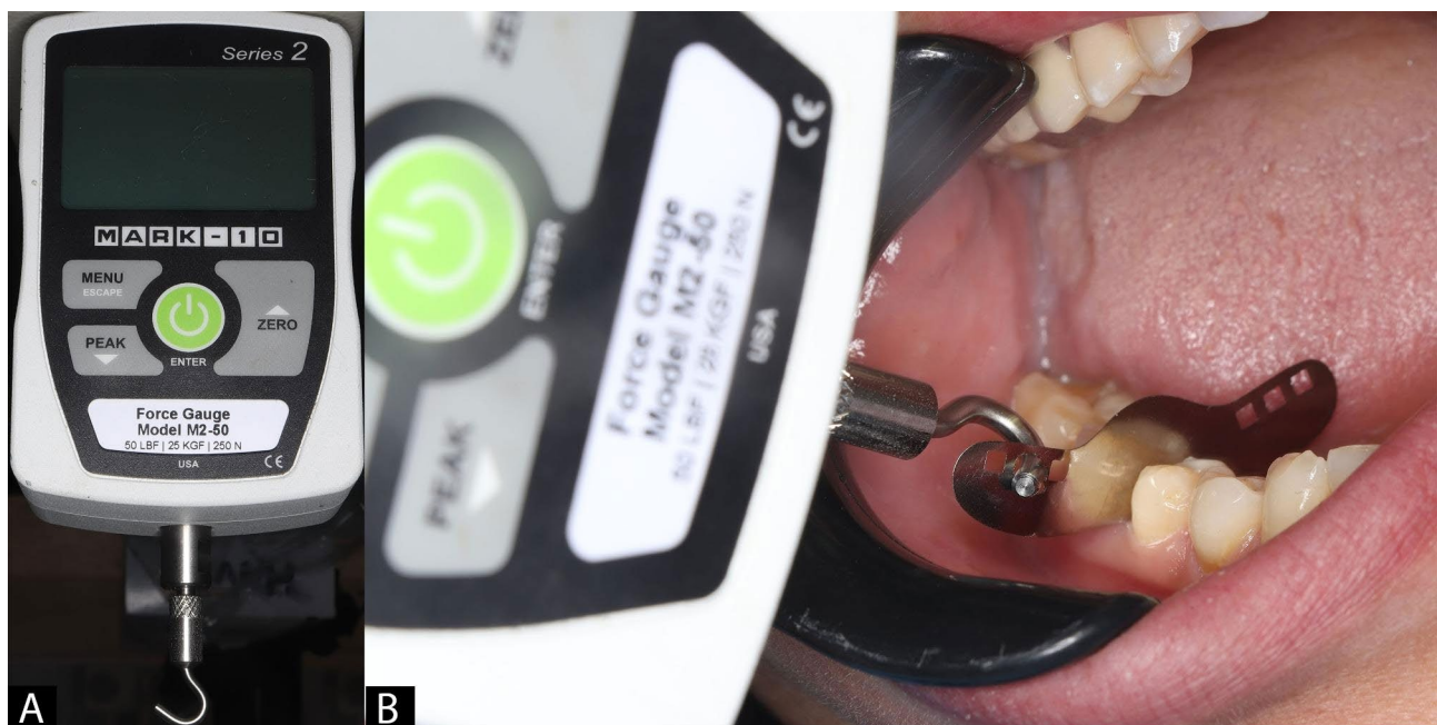
Fig. 2 Showing (A) Mark-10 series 2 digital force gauge with small hook, (B) pulling of 0.05 ivory sectional matrix from buccal direction
