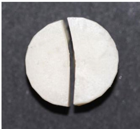
Fig. 2 The fractured bilayered composite-zirconia specimen
