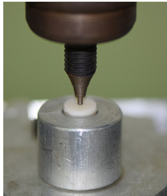
Fig. 1 Load-to-failure test of samples using universal testing machine showing the piston touching the tested specimen
