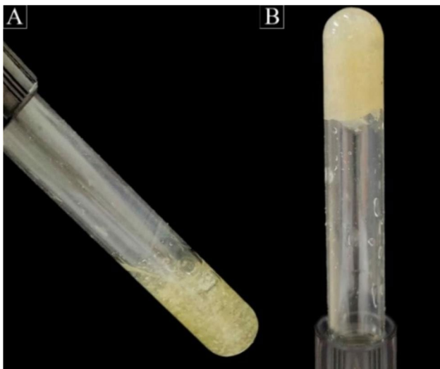
Fig. 2 Example of a gelation time measurement by inverted vial method; (A) TDMH before crosslinking; (B) TDMH after crosslinking with \text{CaCl}_2
