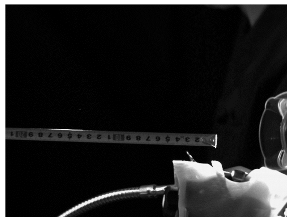
Fig. 3 Images taken by the high-speed camera (calibration data). Each image was taken with an angle of view of 640 × 480 pixels, and the actual size of one pixel was 0.45868 mm
