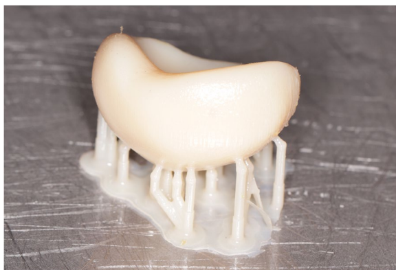
Fig. 3 3D-printed ocular prosthesis using medical grade 3D-printed acrylic resin (Preform; Formlabs, USA)
