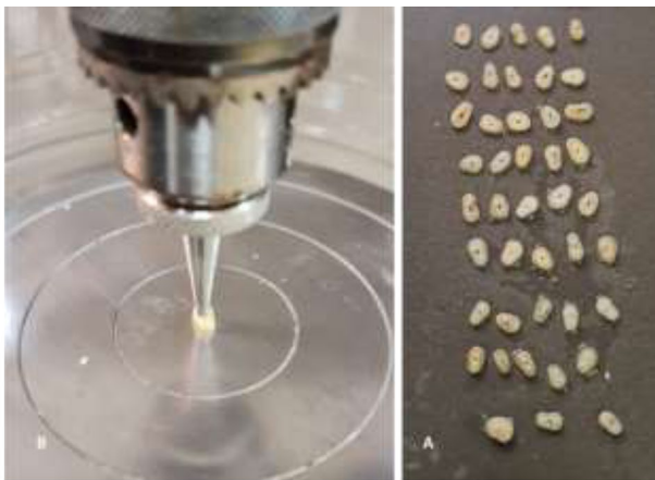
Fig. 2 (A) Dentinal disks from one of the experimental groups undergoing compressive strength testing (B)
