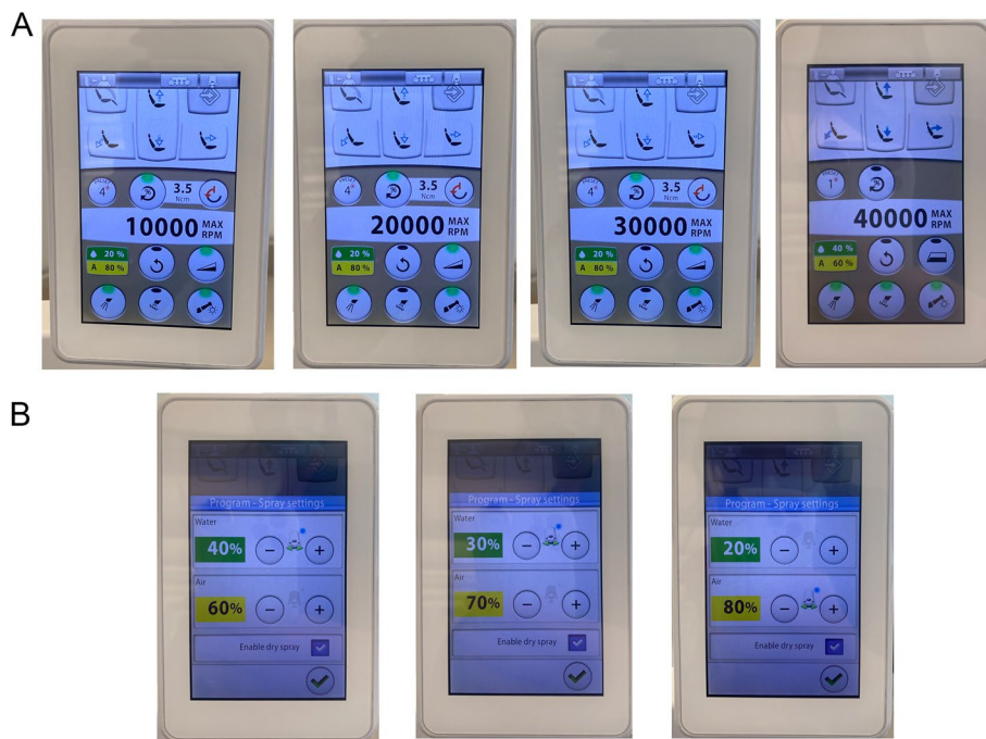
Fig. 4 Digital dental unit with control panel where dental handpiece speed (A, top) and cooling condition (B, bottom) can be adjusted
