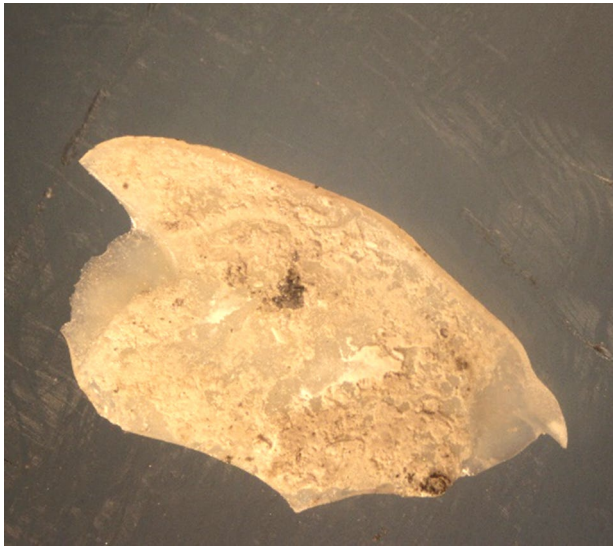
Fig. 5 A fragment of a broken debonded LiSi occlusal veneer
