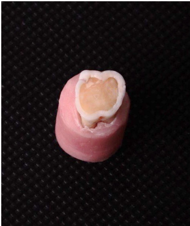
Fig. 1 Tooth after preparation. Central dentin and circular enamel was exposed peripherally to simulate a worn occlusal table
