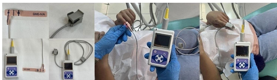
Fig. 2 Measuring finger SpO 2 value using PO infant probe and finger probe
