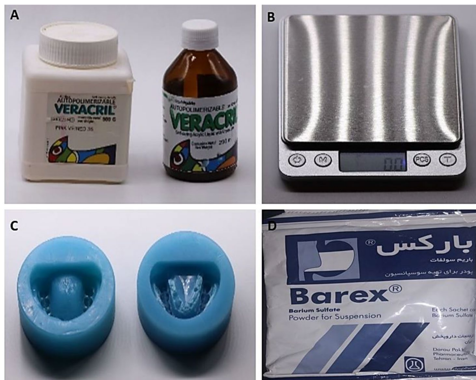
Fig. 2 Materials for Cast construction indicating Veracril (A), sensitive balance (B), mold (C), and Barium sulfate (D)
