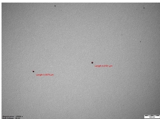
Fig. 1 The TEM image of silver nanoparticles in NSF solution (1 \mu\text{m} = 1000 nm)
