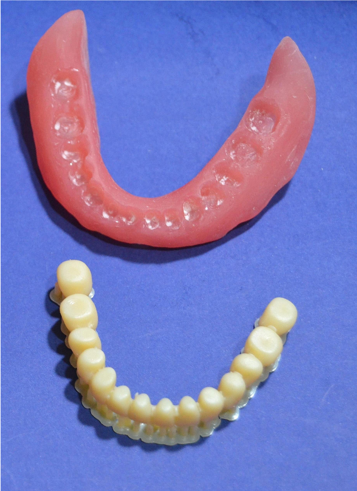
Fig. 4 3D-printed denture base and teeth immediately after printing and before bonding
