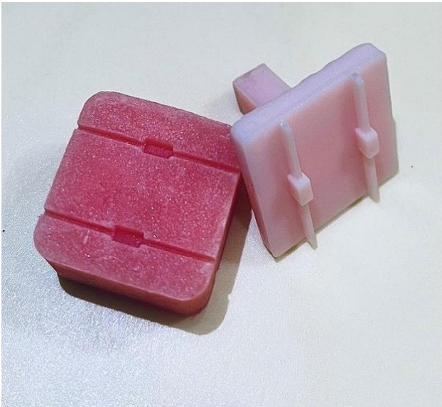
Fig. 5 3D-designed stamp for wire pull-out test
