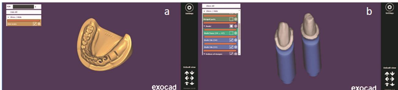
**Fig. 2** a. Diagram showing the virtually designed model having the sockets of abutment teeth and the strain gauge slots. b. Diagram showing the virtually designed abutment dies having a heavy chamfer finish line
