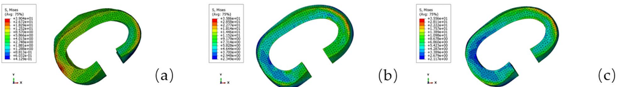
Fig. 13 Cloud of stress distribution in the enamel layer of different restorations under oblique loading: (a) endocrown ; (b) ; inlay crown; (c) post core crown
