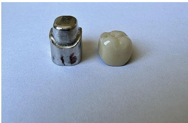
Fig. 2 CoCr die model fabricated by CAD/CAM milling
