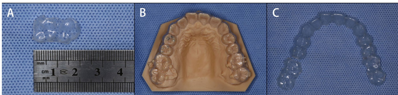
Fig. 5 Fractured pieces of the orthodontic invisible aligner. (A) 2-centimetre swallowed piece of the aligner; (B) Fractured pieces of the whole aligner on the 3D-printed model; (C) Fractured pieces of the whole aligner
