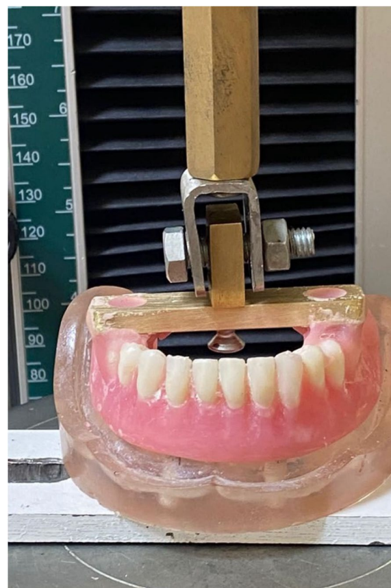
Fig. 14 Metallic cobalt-chrome bar attachment with grasping hook in the middle of the bar was fabricated to engage the denture and facilitate the application of the tensile load
