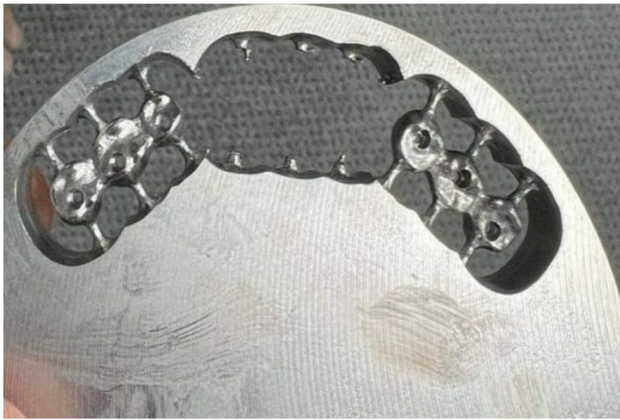
Fig. 3 Milled 3-unit implant supported framework from cobalt chromium block
