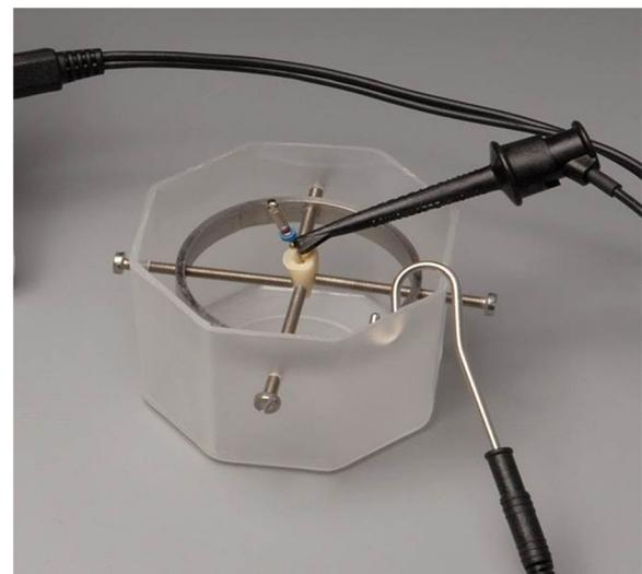
**Fig. 1** Experimental setting with tooth fixed for detecting the apical constriction. The roots were covered with 0.9% NaCl solution
