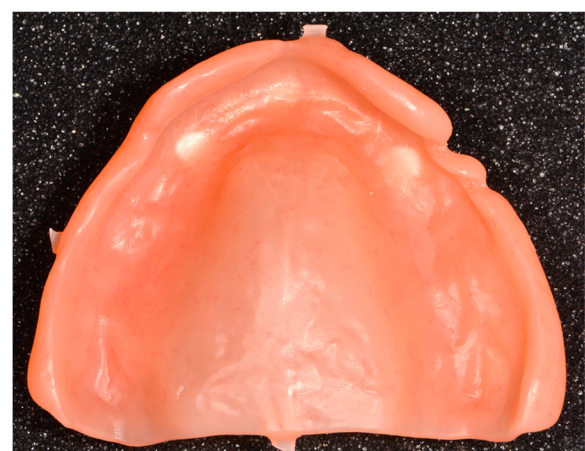
Fig. 32 Once the bonding is complete, the disc is put back into the machine to mill the denture intrados. If a prosthetic tooth base interferes with the virtual model, it will be machined according to the correct intrados
