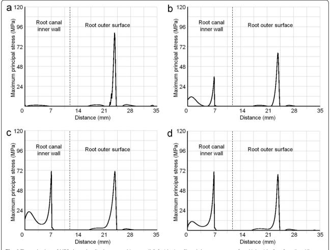
**Fig. 4** The path plots of MPS along the distal root canal inner wall (left side,  $1 \rightarrow 2$ ) and the root outer surface (right side,  $2 \rightarrow 3 \rightarrow 4$ ). **a** All types of endocrown; **b** GF post; **c** SS post; **d** MC post. The left peaks in **b**, **c** and **d** were caused by the post tip, the right peaks were caused by root furcation area
