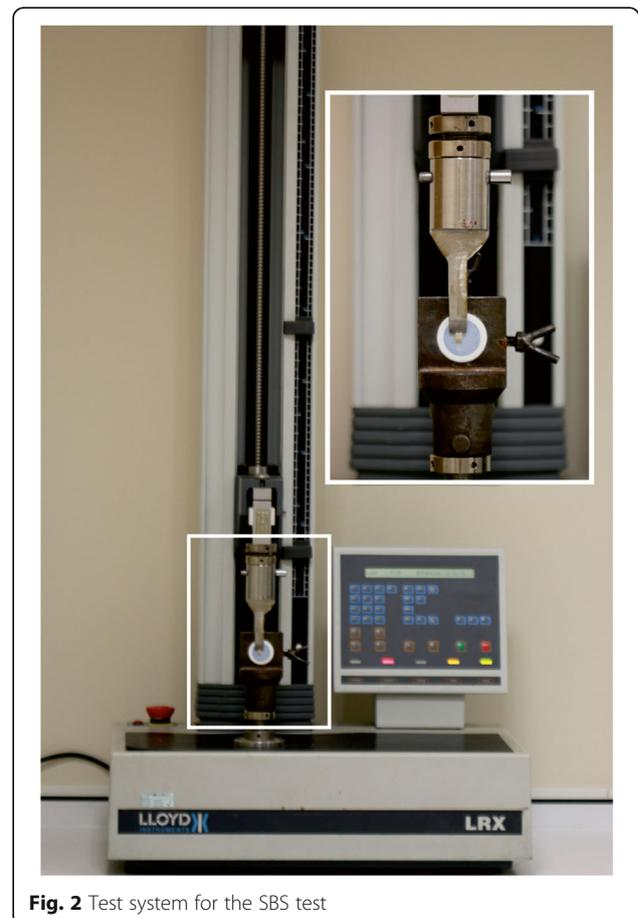
**Fig. 2** Test system for the SBS test
